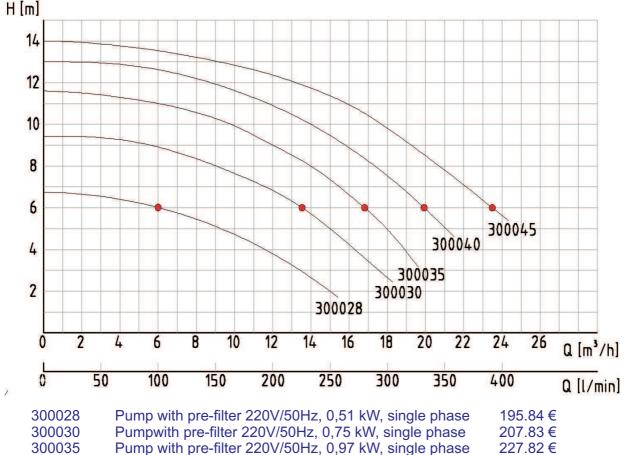
Pump with pre-filter 220V/50Hz, 0,97 kW, single phase Pump with pre-filter 220V/50Hz, 1,3 kW, single phase 300040 307.75€ Pump with pre-filter 220V/50Hz, 1,71 kW, single phase 300045 355.72 €
