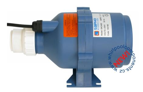
**150180** Blower SAC400, 400W, 230V/50Hz N=23 000 rev/min cable 2m, union 32mm
